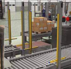
A palletizer can be very dangerous for nearby operators, especially when they must access the pallet after the robot is finished. SG4 Body Compact with pre-mounted, pre-cabled and pre-aligned muting arms fulfils completely this requirement reducing installation costs without jeopardizing the safety level.
