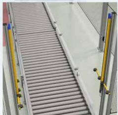
Palletizing cells require protection around the entrance and exit to allow for the detection and prevention of injuring a nearby operator.
