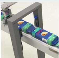
The HFFS machines operate on continuous cycle, taking the plastic wrap from a reel and sealing it around the product. The Area Sensor is used to detect different objects. inside the plastic wrap.
