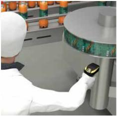
When loading the wrapping material into the machine, operators have to double check they have selected the correct one. This verification can be automated by using an industrial handheld reader like the Powerscan.
