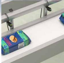
The HFFS machines operate on continuous cycle, taking the plastic wrap from a reel, sealing it all around the product. BKGD suppression or polarized sensors are typically used to detect the material on the belt.
