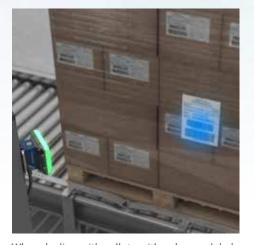
When dealing with pallets with unknown label position, a very powerful scanner is needed for barcode reading. Thanks to the high imager resolution and extremely powerful lighting system, Matrix 450N delivers high reading rate on wide Field of View and extended Depth of Field.
