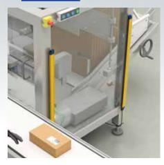
Light curtains allow safe entry to potentially dangerous operations. The ideal hazardous point protection involves minimizing ergonomic restraints and maximizing secure detection. SLIM Safety light curtains fit perfectly into the machine frame even when very little space is available.
