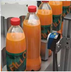
Label check is a typical need in labelling machines to prevent issues such as missing labels or mis-labelled products. The DataVS2 vision sensors are able to reliable detect these production errors and can be quickly programmed by non-expert users thanks to the easy-to-use Graphical User Interface.
