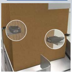
The Automatic case-packers are used to solve the works of forming, loading and sealing of cases. Photoelectric sensors are used to verify the presence and the position of the cases in order to guarantee the right process.
