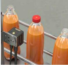
In the filling machines a quality issue is the verification of the presence of the bottles cap. The Smart-VS vision sensor is the most suitable solution for this verification.
