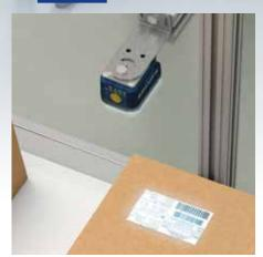
Single packages are often grouped into bundles. In order to ensure the traceability of products, labels with barcodes are usually applied on bundles and have to be read automatically. The Matrix 300N, features a 2MP high resolution imager and powerful lighting system, allowing it to read barcodes over a wide field of view.
