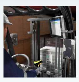
The PowerScan 2D Auto-Range ensures high reading performances of both 1D and 2D codes even at far operating distances. Combined with the SD9030 dongle and the Rhino II vehicle mount computer, it represents a complete solution for forklifts allowing operator to scan items with no need to get off the vehicle.
