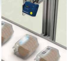
F&B customers typically have to manage a very wide range of products on the same manufacturing line featuring different graphics according to the flavour, language, brand, etc... Matrix 120 is an extremely compact reader that can be embedd into any space of the machine to verify the correctness of the packaging material.
