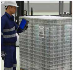
Inventory management requires periodic verification of the goods stored in different locations. The Taskbook, a rugged tablet with optional handgrip that integrates a 2D imager and a hot swappable battery, represents the most efficient solution for tracking allowing one hand scan on 24/7 basis.
