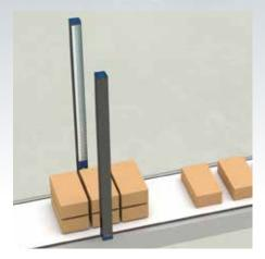
In the automatic case-packers a quality issue is the verification of the bundle completeness before the insertion of it into the case. Light grid system is used to measure the height of the bundle in order to verify that the right number of packages are wrapped and ready to be inserted into the case.
